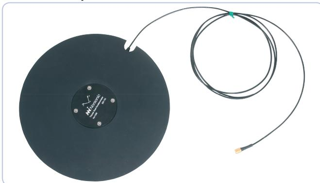
This triaxial seat accelerometer is designed for whole body measurements according to ISO2631 and ISO8041. The integral cable is 2m and the connector fits the Nor133 and Nor136 vibration meters. The seat pad consists of a rubber pad, an aluminum mounting adapter plate to where a triaxial accelerometer type Nor1288 is mounted. The Nor1288 accelerometer port is detachable for calibration purpose.
